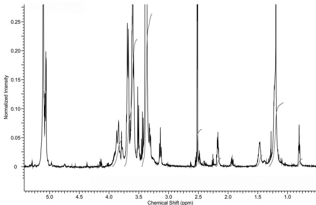
Fig. 1.  $^1\text{H}$ NMR spectrum of starch oleinate.
