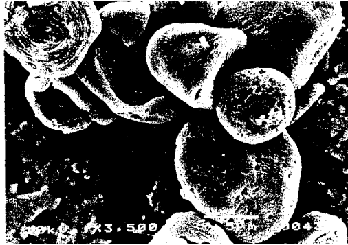
Fig. 4. Maize starch after enzymatic modification.
