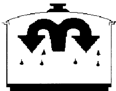
Schładzanie i skraplanie pary Cooling and condensing of steam
