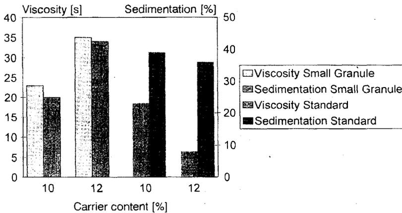
Fig. 5. Viscosity and sedimentation of Stein-Hall type corrugated board adhesive.
